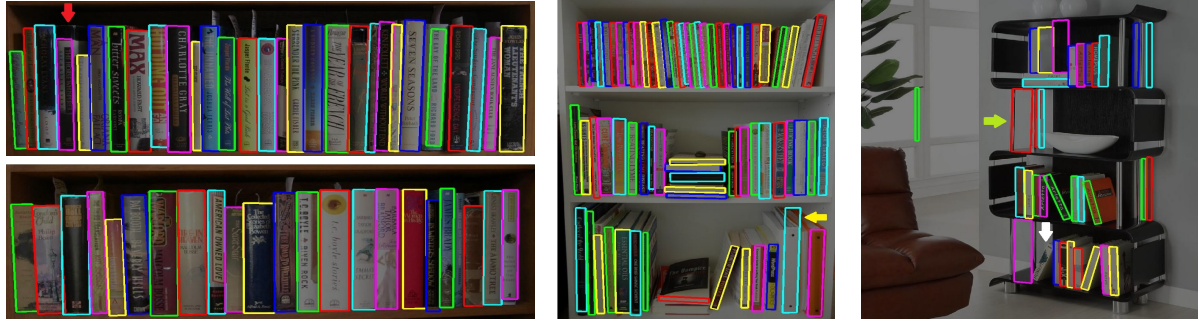
Figure 7: Book spine segmentation results and typical segmentation errors. Left, dataset 1; middle and right, dataset 2. Arrows mark segmentation errors: overextension (yellow); partial segmentation (red); false negative (white); false positive (green).
